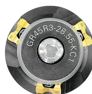
fig. 45°-bevel-milling head with 3 cutting edges and guide roller, equipped with 3 bevel-indexable inserts of type K
